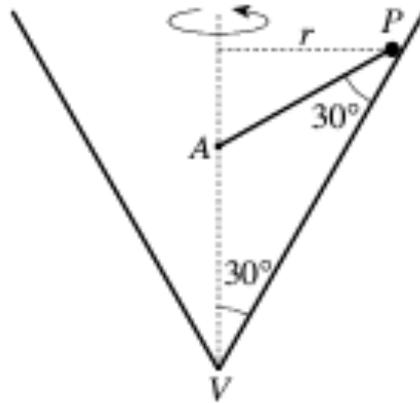
A hollow circular cone is fixed with its axis vertical and its vertex  $V$  downwards. A particle  $P$ , of mass  $m$  kg, is attached to a fixed point  $A$  on the axis of the cone by means of a light inextensible string of length equal to  $AV$  metres. The particle moves with constant speed  $v$  m/s in a horizontal circle on the smooth inner surface of the cone, with the string taut. The radius of the circle is  $r$  metres, and angles  $APV$  and  $AVP$  are each  $30^\circ$  (see diagram)
